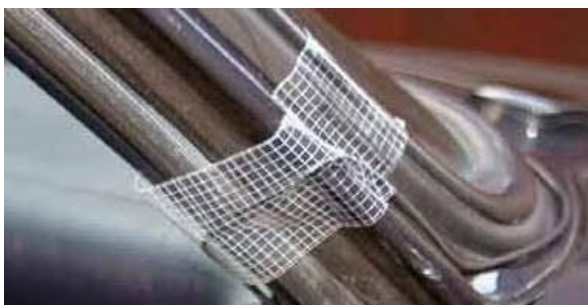
Passage câble antenne / e.g. Antenna's cable sitting
